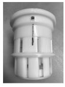
When reassembling the register parts before installing into the meter, line up the alignment indicator on the register with the line drawn on the rotor housing,
