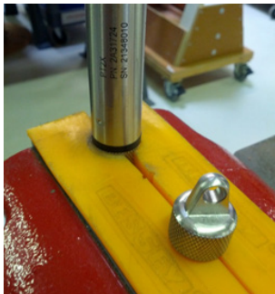
Cableless Sensor—gripping on knurled area
