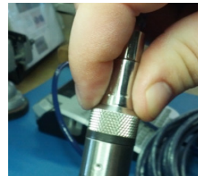
Properly completed—black ring uncompressed
