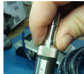
Properly completed—black ring uncompressed
